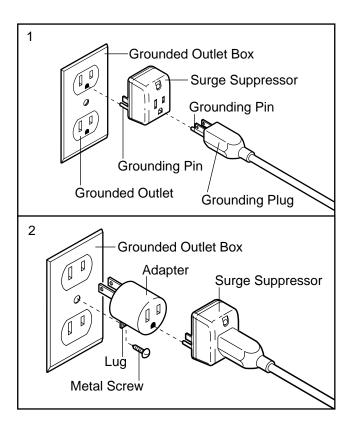
The green-colored rigid ear, lug, or the like extending from the adapter must be connected to a permanent ground such as a properly grounded outlet box cover. Whenever the adapter is used it must be held in place by a metal screw. Some 2-pole receptacle outlet box covers are not grounded. Contact a qualified electrician to determine if the outlet box cover is grounded before using an adapter.
